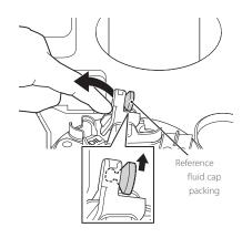
c. Wipe off the reference fluid cap using a cotton swab or soft cloth moistened with distilled water. Dry it after cleaning.
