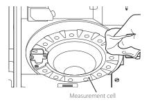
i. Loosen the 2 screws on the reference plate and remove the plate from the analyzer.
