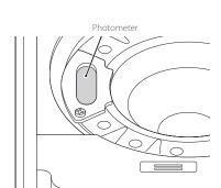
l. Replace the reference plate. Tighten the 2 thumbscrews evenly.
