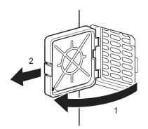
3. Remove dust adhering to the filter with a vacuum cleaner or running water. **NOTE:** If washing the filter with running water, make sure the filter is dried well before placing back into the analyzer.
