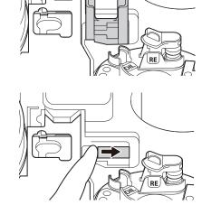
d. Air blow from the gap where the slide cartridge is placed, as shown in the figure.
