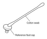
d. Replace the reference fluid cap properly. NOTE: Do not touch the bottom (reference fluid side) of the reference fluid cap.
