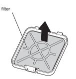
4. Insert the filter into the louver and put the louver back on the analyzer. Insert the back side of the louver first, then snap the front side in place.
