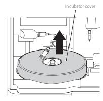
e. Loosen the 5 screws on the upper surface of the incubator, and then remove the incubator.
