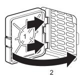
Remove dust adhering to the filter with a vacuum cleaner or running water. NOTE: If washing the filter with running water, make sure the filter is dried well before placing back into the analyzer.
